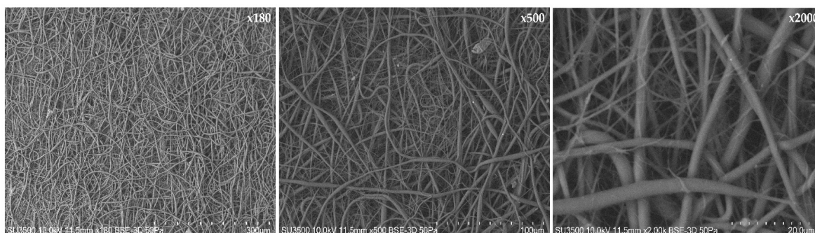
Figure 4. SEM of electrospun PCL/PEO dc-AgNP nanofibers at ( \times 180 ), ( \times 500 ) and ( \times 2000 ) magnifications.
